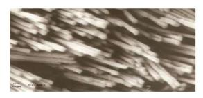
Fig.8 SEM Photograph of copper nanowires of 200nm diameter grown by electrodeposition in AAM<sup>15</sup>.
