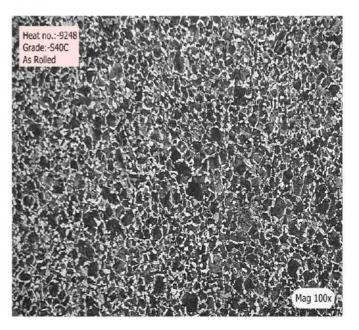
Fig. 3.4 Microstructure of As Rolled Sample
