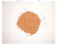
Figure- Alumina Slag as strengthener Research and development work on Alumina Slag utilization that are under process in India are shown in table no.3. Going through the available information on the utilization of Alumina Slag (density 3.05 g/cm3) [6], it is seen that use of Alumina Slag as strengthener material for preparation of MMC has not been explored till date [1].
