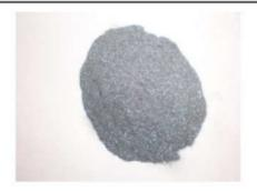
Figure- Silicon Carbide (SiC)
